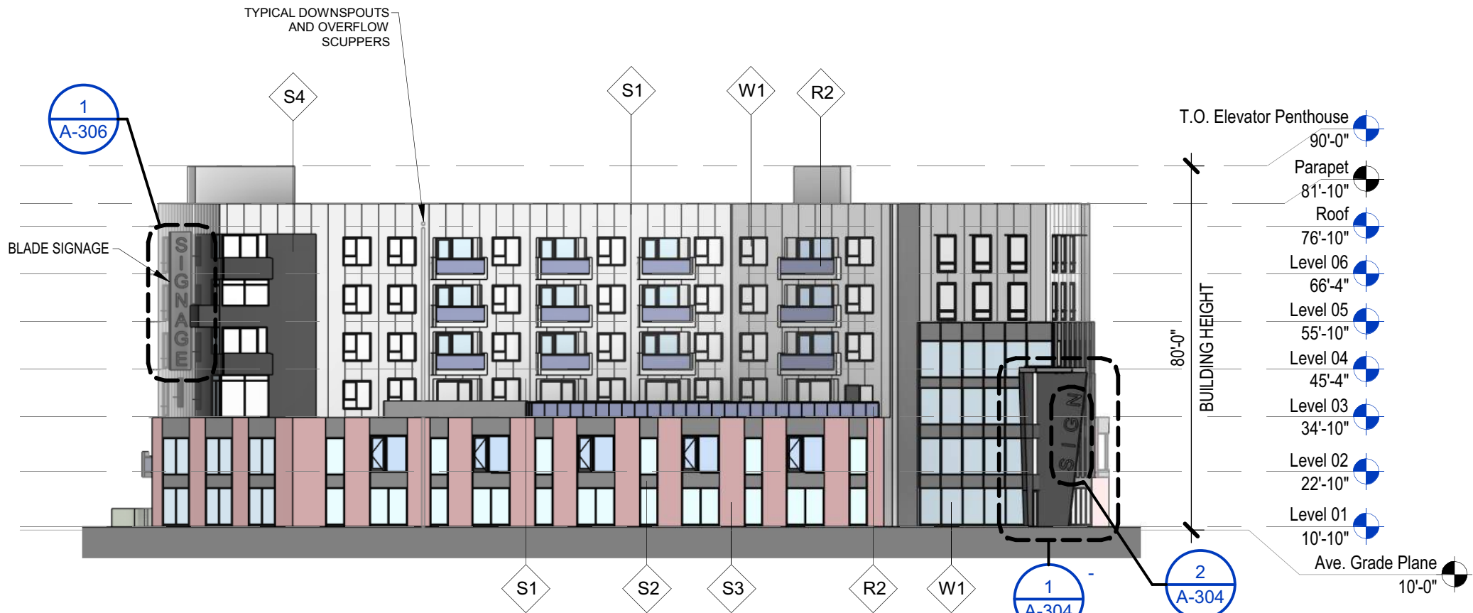
BUILDING NORTH ELEVATION
